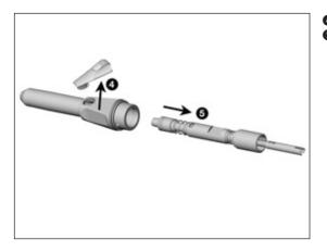
4 Remove the chuck lever.
