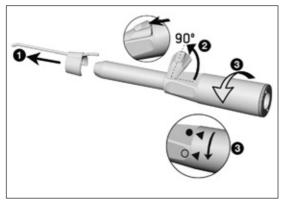
Disassembling the straight medical device S-11, S-15
