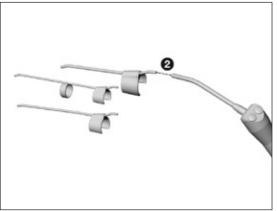
Blow through the coolant tube and coolant outlets using compressed air.
