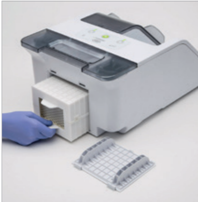
Twin Care Set Each set comprises one cartridge of cleaning solution, one cartridge of Service Oil F1 and one HEPA filter. All consumables are extremely easy to replace without a tool.
