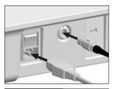
Connect the mains cable and wired foot control (only for SI-2100).
