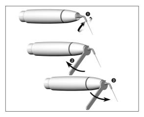
Insert/remove tip with spanner
