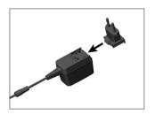
• Attach the adaptor to the power supply unit.
