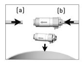
Replace the air filter and reconnect the air hose (a, b).
