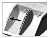
Close one chamber using the sliding window.
