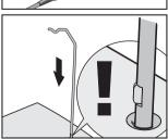
Insert the irrigant support. Pay attention to the positioning! (maximum load capacity 1.5 kg)
