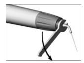
• Unscrew the tip using the spanner.
