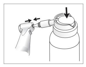
Lubrication of the chucking system WE-99 LED G
