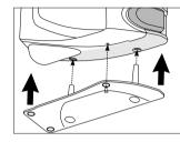
• Assemble the control unit onto the foot stand with compressed operating panel (control unit with internal coolant supplying).
