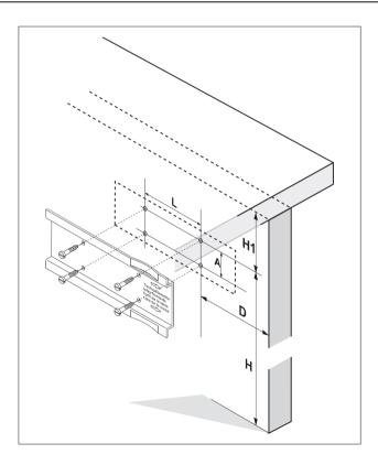
• Mark the screw holes with the enclosed drilling template or holding plate.
