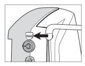
• Push in the fitting for the blow out function up to the limit stop.
