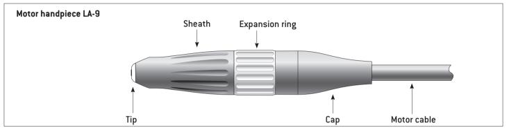
The milling device adaptor (optional) for the motor handpiece can be fastened above or below the expansion ring. The milling device adaptor (optional) has a diameter of 16 or 18 mm on either side for use with different milling devices.
