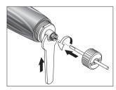
Insert the chuck key up to the limit stop in the chuck and unscrew anticlockwise.
