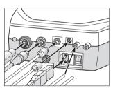
Connect the motor cable, operating controls, foot-operated starter, air hose, coolant hose (control unit with external coolant supplying) and mains cable.
