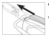
Insert control unit up to the limit stop on the holding plate.
