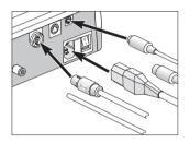
• Connect the motor cable, operating controls (optional), air hose (Perfecta 600) and mains cable.
