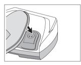
You can switch between forward and reverse operation by pressing the button.
