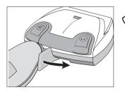
By activating the foot lever, the values 1,000 – 40,000 rpm (1,000 – 50,000 rpm with Perfecta 600) are continuously increased / decreased.
