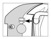
Push in the fitting for the blow out function up to the limit stop. (Perfecta 600).
