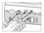
Connect the motor cable, operating controls, footoperated starter, air hose (Perfecta 600) and mains
