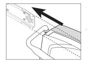
Insert control unit up to the limit stop on the holding plate.
